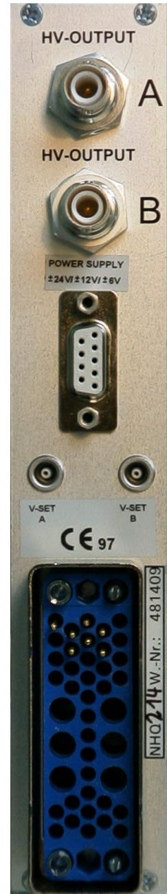
Figure 5.3: 2x4kV Power Supply (rear-panel)
